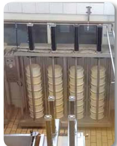
Figura 57. Prensa vertical manual
