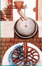
A model of a cross-section of the mill explains how the water makes the grindstones work, thereby obtaining flour from the grain.
