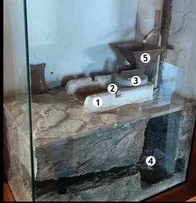
**5** The «Tolva» or hopper is a type of big wooden funnel or trough that spreads the grain over the grindstones at a constant rate.
