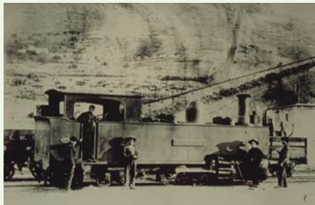
Locomotive LUCAINENA (Nasmyth Wilson 464/95), one of the machines used on the mineral transport line from Lucainena to Agua Amarga. The photo dates from the end of the 19 th century (Photo, Col. J.M. Sánchez Molina).
