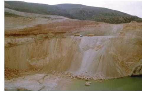
Los Trancos quarry is the principal bentonite mining concern in the park. The extent of the quarry benches can be observed, taking the lorries as a scale.
