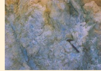
Bluish and greenish colouration corresponding to superficial alteration minerals of copper and lead sulphides.
