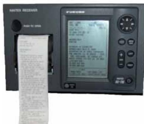
Figura 1. Foto receptor NAVTEX
