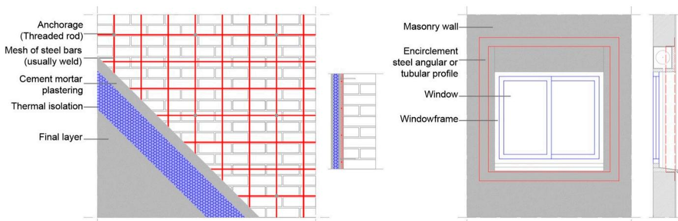
**Figure 10.** Conceptual details of the retrofitting packages: wall strengthening and addition of thermal insulation and addition of encirclements and window replacement/enhancement.
