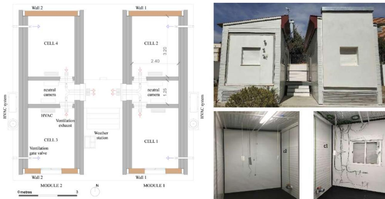
Fig. 1 Floor plan and images of the test cells.
